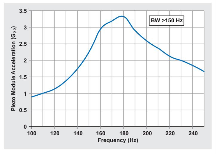
**Figure 6. Acceleration characteristics of an LRA**
